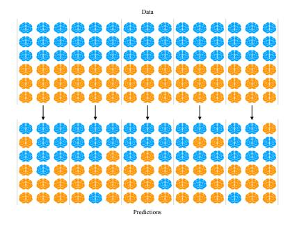
At this point we can compute accuracy as the fraction of correctly classified samples. In this example we have 11 misclassified points (79 correctly classified) out of 90, producing an accuracy of 88%.
